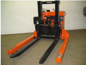
The walkie style pallet stacker is the most commonly used of all electric powered pallet stackers. Pallet stackers are similar in design and function to [counterbalance lift trucks](#) but have many additional functions and advantages.
